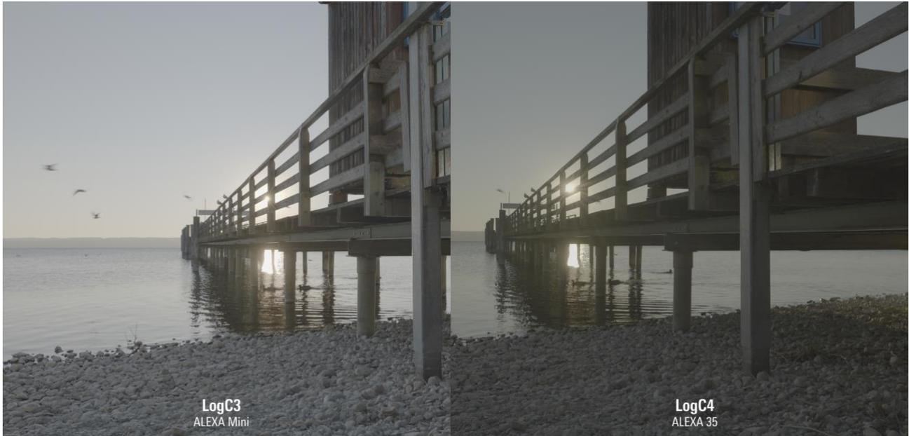
LogC4 is very different from LogC3 (the Log C you are used to)! This calls for adaption when exposing the sensor as a single operator as well as for DITs who monitor exposure or do live grading. **LogC3 3D LUTs do NOT work with LogC4 and may lead to unwanted results!**
