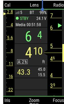
The Hi-5 hand unit is compatible to the L-Series battery interface and works with respective 3rd-party batteries such as NP-F550 type batteries. However, there is no accurate capacity display with these batteries and the hand unit can shut off abruptly without warning.
