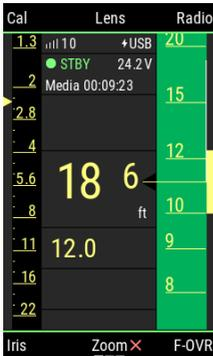
Return focus control to Hi-5 on the OCU-1/Master Grip or by pressing the F-OVR button on the Hi-5. The Hi-5 focus scale turns green. The focus knob is still offset (see motor trail at the currently set motor position).
