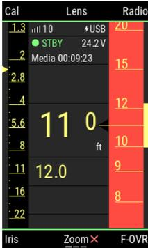
OCU-1/Master Grip overrides focus control from Hi-5. Hi-5 focus scale turns red. Hi-5 has no control over focus axis.
