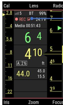
Pressing the REC button briefly during recording in tail-slate mode will not stop the recording, but generate a warning that tail-slate mode is active.
