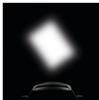
The framing module is rotatable by +/- 65°
