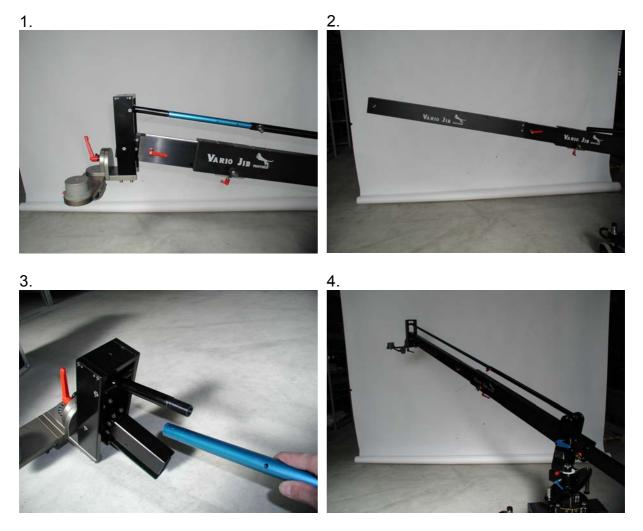
The Extension is mounted between the telescopic tube and the end-section. Take off (unscrew) the blue leveling rod and extend it with the extension rod. The second counterweight rod is put into the second hole of the back outrigger and loaded.
