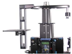
The running board bracket gives the cameraman the possibility to be moved with the column (in combination with a platform and seat extension). The running board bracket is mounted onto the turnstile. Please take off the bolt on the shorter side of it.
