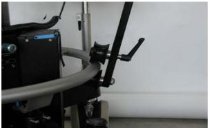
**3.2 Connecting rod** The connecting rod is mounted to the ring. The wheels grasp the ring.
