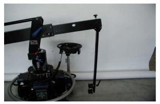
**3.1 Connecting rod** Screw the connecting rod onto the back outrigger of the Vario Jib.
