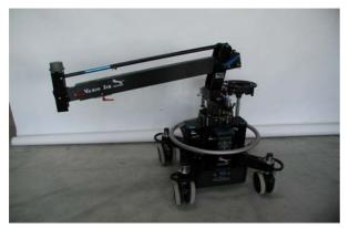
**2. Vario Jib** Put Vario Jib onto Euroadapter and tighten screws. The Turnstile is turned 90°.
