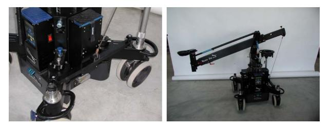
The Jib cable can be used instead of the Jib A-Round-Kit. It is mounted to the back outrigger and on two wheel arms.
