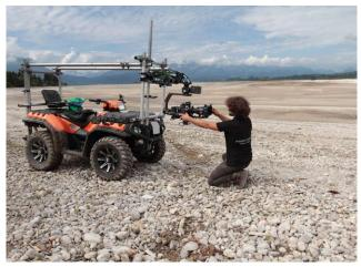
IDEA VISION GmbH Anzengruberstr. 16 83059 Kolbermoor D-Germany There are several ways to attach your gimbal to the Hybris shock absorber. The included plate has hole base patterns to match the Freefly Toad in a hole and Cinemilled Universal Ronin mount for easy attachment of the MoVI and Ronin gimbals. We also make a Mitchell female mount for gimbals that uses the Mitchell connector.
