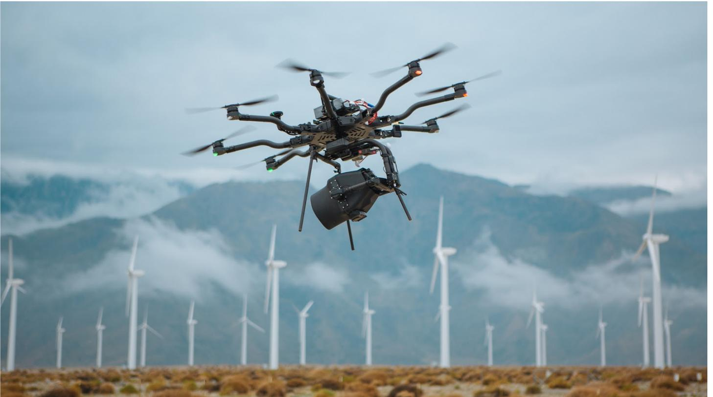
ALTA Pro is a professional multi-rotor aircraft designed for demanding cinematic, professional, and industrial, applications. In under five minutes, ALTA Pro can unfold from its carrying case to flying some of the most capable cinema cameras and industrial payloads on either the top or bottom of the aircraft. ALTA Pro runs the PX4 stack and has been customized for both cinema and commercial use, yielding precise yet smooth control.
