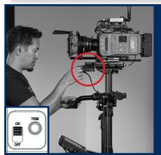
IF the control box is mounted for goofy operators (knobs on the LEFT) align the gimbal handle with the FRONT of the post and simultaneously power on the Volt. Wait 2.5sec while the system registers the pan encoder position.
