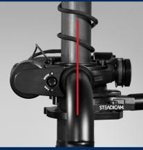
**REMEMBER:** If your box is mounted with the knobs to the RIGHT (regular), you'll align the gimbal handle to the REAR when powering on later.
