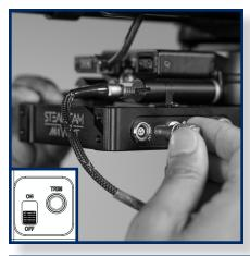
Ensure the power switch is in the OFF position and connect the short power cable from sled power to the 12V IN port.
