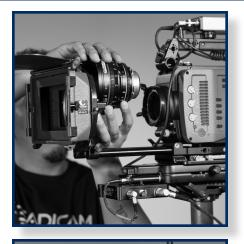
When changing accessories above the gimbal, like lenses or filters, re-balance on the pin with a normal drop time and then go fully neutral again.
