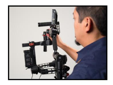
If necessary, go back and re-center the Steadimate using the Tilt Balance Knob as previously described on page 4-2 of this manual.
