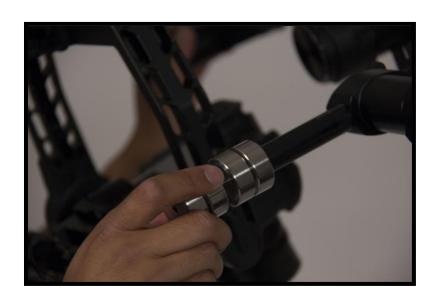
With the Post Block height set correctly, you can later add or remove weights when accessories, lens swaps or personal preference require small, quick changes to the CG of the system.
