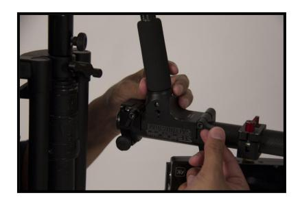
Turn the Tilt Balance Knob one way or the other until the handle stays vertical.
