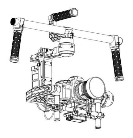
With the motorized gimbal resting on the tuning stand, remove the right side handle.
