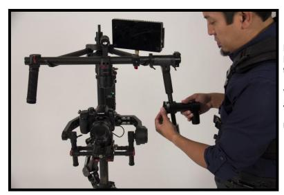
Loosen the Post Clamp and slide the Post Block one number down the Post scale and retighten the Post Clamp.
