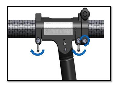
Tighten the Handlebar Clamp Locks by hand and securely tighten the Tilt Balance Lock Screw with the included 4 mm Allen key.
