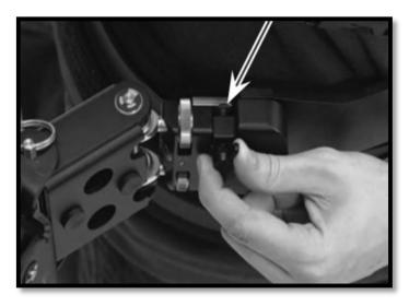
If the rig tends to move straight away from you; loosen the bottom Thumbscrew and tighten the top Thumbscrew until the rig is neutral. Then re-tighten the bottom Thumbscrew.
