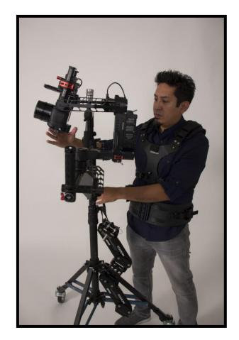
While still on the Balance Pin, hold the Steadimate handle vertical and loosen the two Handlebar Clamp Locks.
