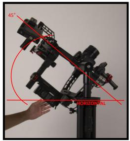
If the Steadimate is truly inverting, where the Handlebar is below the Post Block, then you must balance in Inverted Mode.
