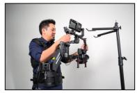
With the tuning stand raised so the Handlebar of your motorized gimbal is roughly at your chin level, bow to the Steadimate and place the Arm Post into the receiver on the Post Block.
