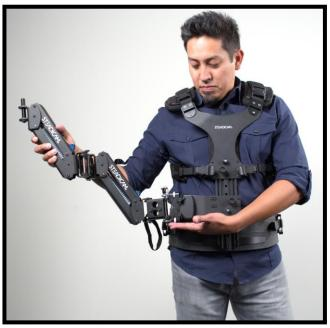
Insert the Arm Socket into the Socket Block of the Vest. Then use the Thumbscrew Bolts to secure the connection.
