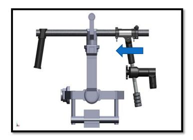
Slide the Steadimate onto the handlebar in place of the handle.
