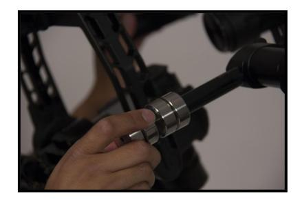
With the Post Block height set correctly, you can later add or remove weights when accessories, lens swaps or personal preference require small, quick changes to the CG of the system.
