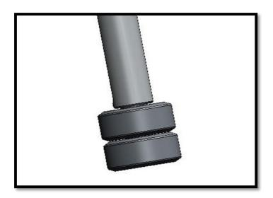
Install **two** Balance Weights at the bottom of the Steadimate Post.
