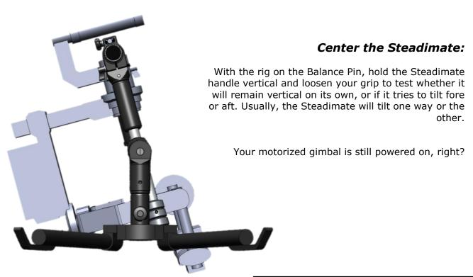
While still on the Balance Pin, hold the Steadimate handle vertical and loosen the two Handlebar Clamp Locks.
