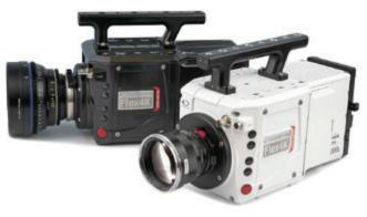
at least 1 millisecond and while it is rare to see the typical distortion associated with rolling shutters, it can still happen when recording subjects with very fast rotating motion. This distortion is eliminated in GS mode, which is also useful to eliminate horizontal bands and vertical scrolling issues when common LED lighting or strobes are present in the scene.
