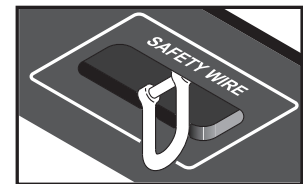
Figure 4: Safety wire attachment point
