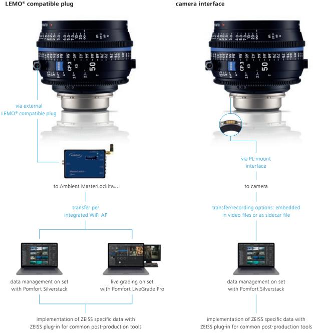
Recording ZEISS eXtended Data via internal camera interface
